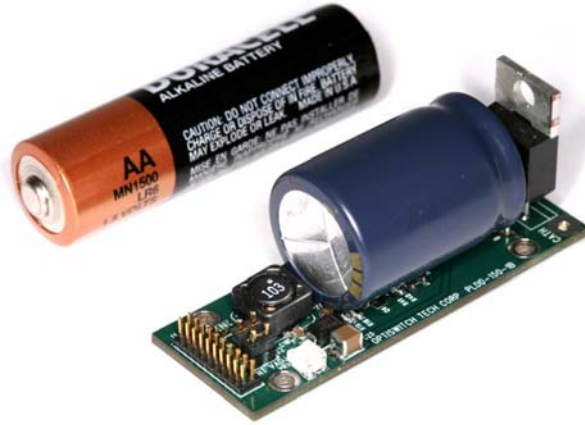
Figure 1. Photograph of the PLDD-150-1-1. This driver weighs 15.2 grams and can deliver 150 amps in 300 \mu s at 1 Hz to a single laser diode from -40 to +70 degC. It can run off a single battery (DL123 or equivalent).
